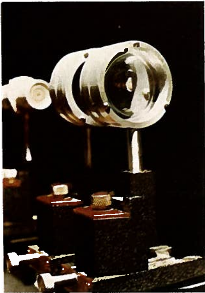
Fig. 2 b—Close-up of the light source and the collimating lenses
